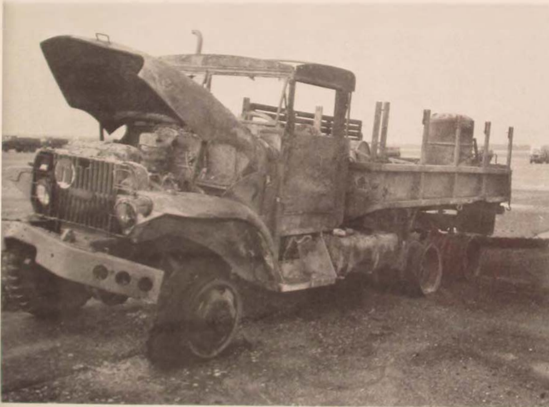
Before the days of high-speed computation, the principal means of evaluating a new munition was by actual test, as on trucks positioned in a target array, with inspection of damage afterward. But tests enough to be conclusive were too expensive, so computers now supplement the test data.
